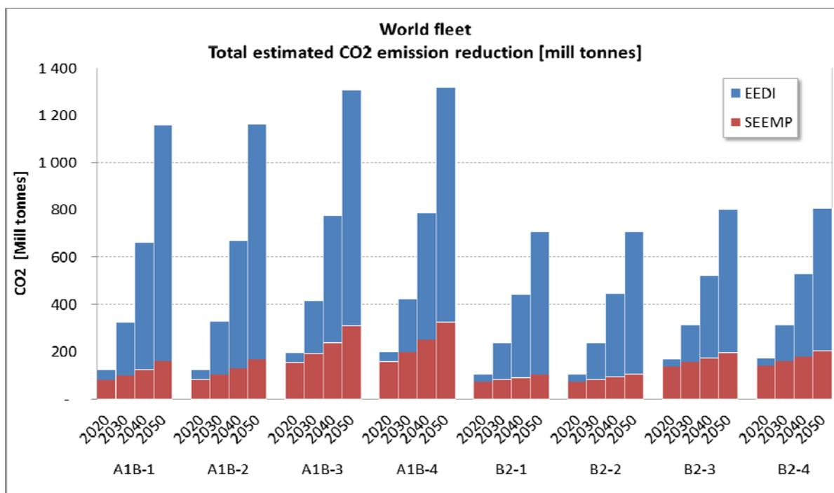
Figure i – Overall annual CO<sub>2</sub> reduction potential for SEEMP and EEDI (waiver 5%)
