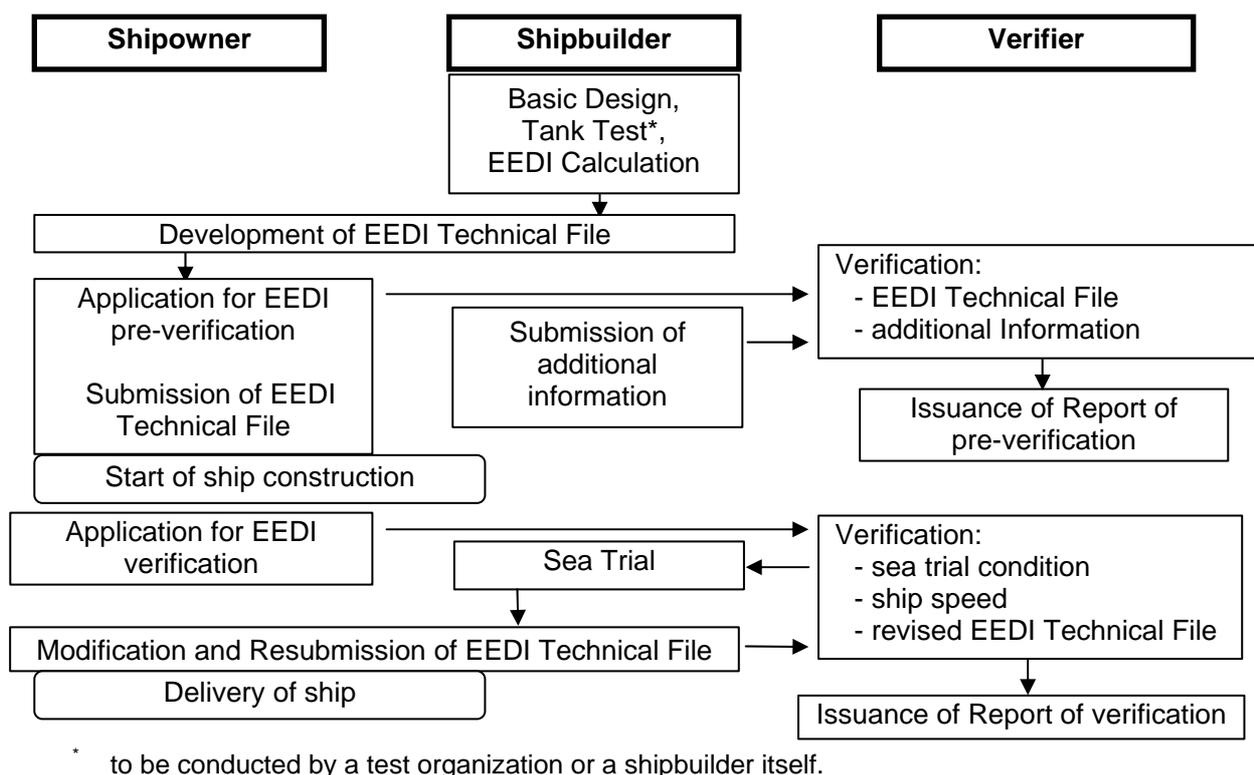
**Figure 1: Basic Flow of EEDI Verification Process**
