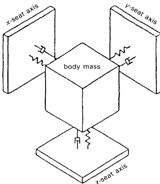
Figure 3 - Independent single-degree-of-freedom representation of human body
