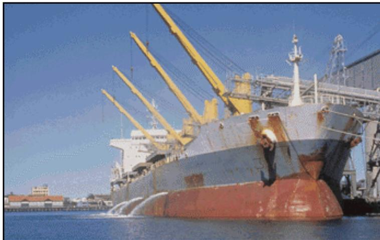
Figure Five: *Routine ballast water discharges from bulk carrier in port (Source: CSIRO Australia)*
