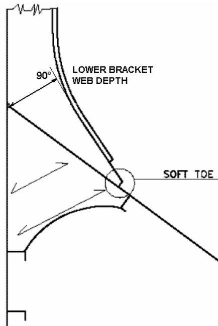
**Figure 4 – Tripping brackets**
