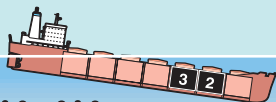
Holds 1 & 2 or 2 & 3: Ship sinks rapidly, no time for crew to abandon ship.
