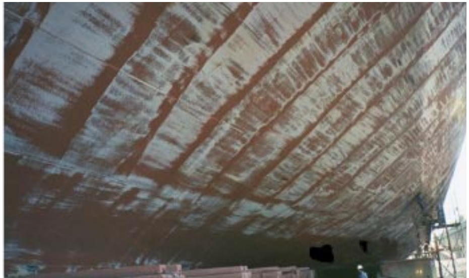
A self-polishing anti-fouling system has been applied to this ship and the polishing pattern that appears when the ship has been sailing for a while can be seen. When applied, all coats appear in red shades. When the outer coat has been polished away and the underlying coat is exposed to seawater it changes to a whitish shade. This allows for monitoring of polishing and performance. The patterns on the hull are the result of overlapping zones arising from the movement of the applicator's hand with the paint gun. (Hempel's Marine Paints)
