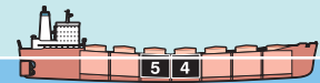
Remaining holds: Sagging, which could cause structural failure, especially if the ship is poorly maintained.
