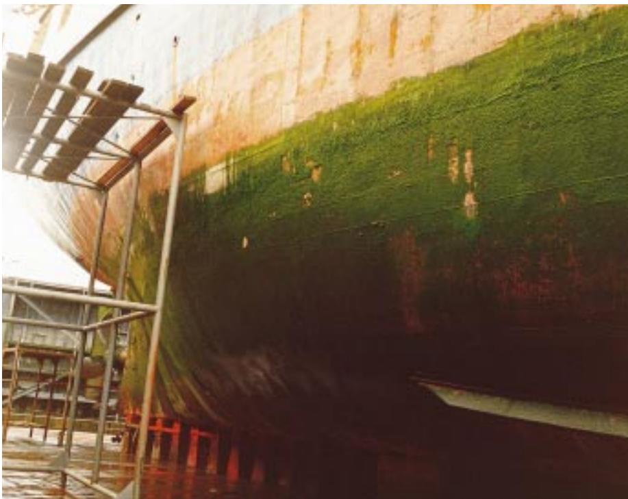
Green algae coats a ship. Just a small amount of fouling can cause a significant reduction in speed and increased fuel consumption. (Jotun Paints)
